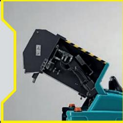
Xtrema is equipped with a polyester bag filter which is particularly efficient for the retaining of fine dust, and has a much longer lasting life than other traditional filters. A highly efficient dust filter-shaker provides extreme cleaning without the need for filter removal.
