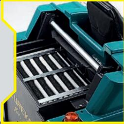
The brush pressure on the floor can be adjusted while working. This is done thanks to an exclusive, precise control positioned on the dashboard
