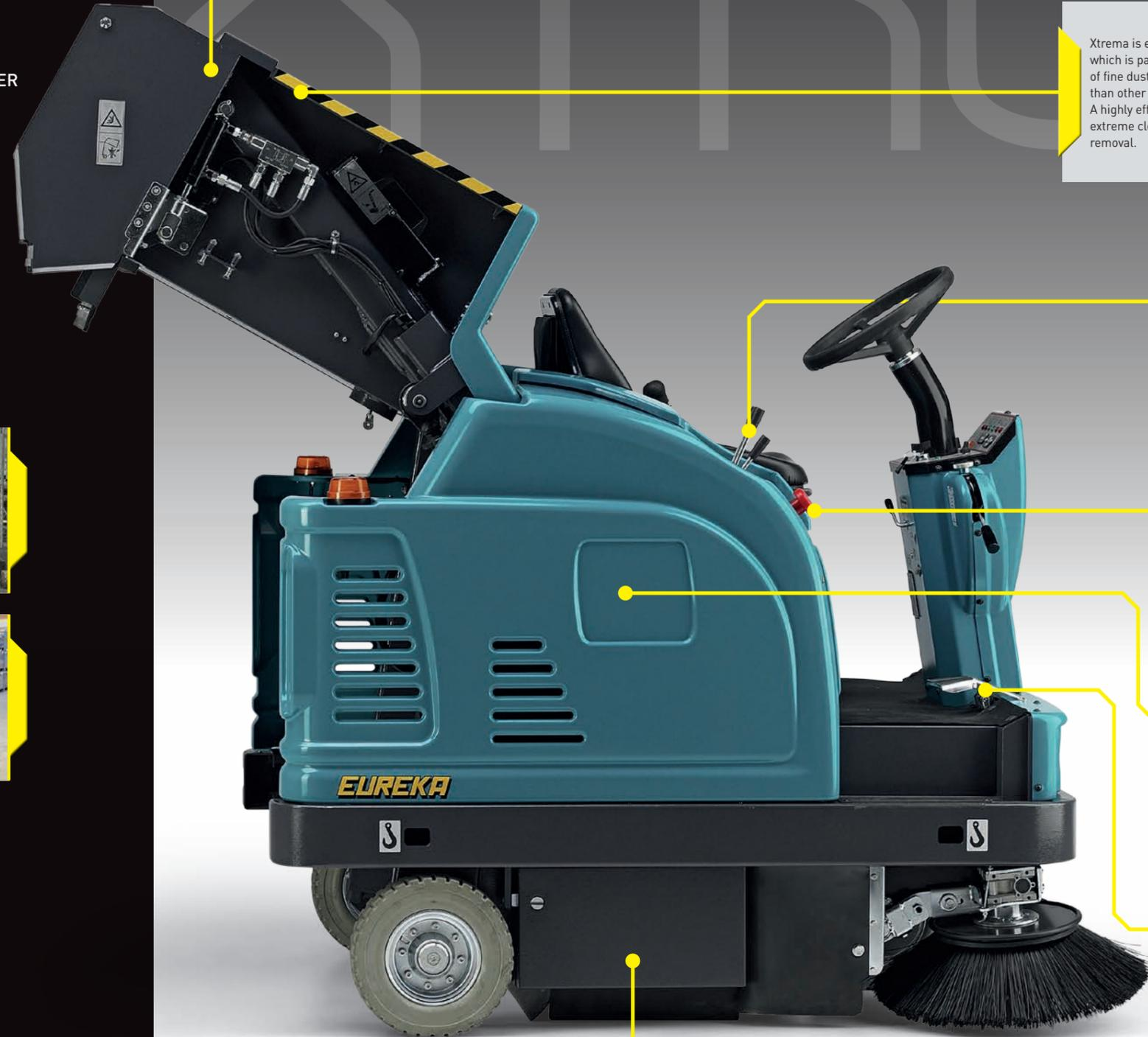
The multi-level-dump hopper, equipped with hydraulic flap, is located in the rear of the machine. It can be hydraulically raised up to 1.360 mm from the floor, and has a volume capacity of 150 litres.
