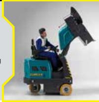
The main brush floats on uneven floors, and automatically adjusts itself when worn. Additionally, the exclusive "Multi Bristle" system enables the main brush to achieve exceptional performances on most floor types.
