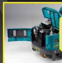
All parts, motors and engines are easily accessible for servicing as side, upper and rear panels can be fully opened. Batteries (EB version) can be replaced easily and quickly thanks to a battery trolley mounted on rolling bearings. This slides out for ease of use.
