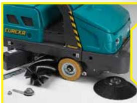
The main and side brush can be quickly replaced without tools.
