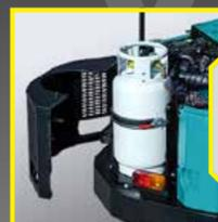
The petrol version is also adapted for use with LPG. It will therefore be possible to work in both indoor and outdoor applications with the same machine.
