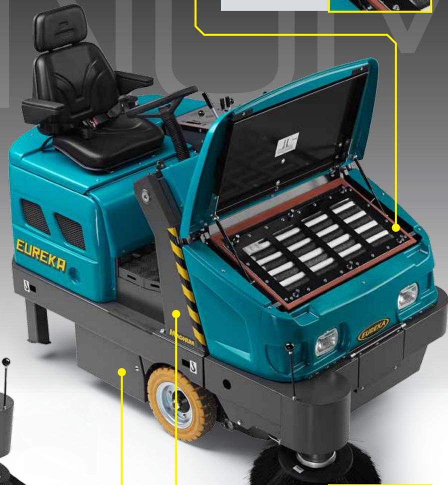
Multi-level dumping system: the hopper, located in front of the machine, can be hydraulically raised up to 1.540 mm from the floor. The hopper is actually floating on the floor, automatically adjusting to allow for easier pick up of larger waste.
