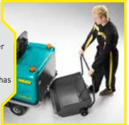
The floating, self-levelling main brush can be quickly adjusted or replaced without need of tools, and the retractable, anti-shock side brushes allow the maximum cleaning efficiency on rough or uneven floors. Integrated in the main brush, which has a width of 70 cm, are: a fine bristle section for fine dust, and a heavy bristle section for larger debris.
