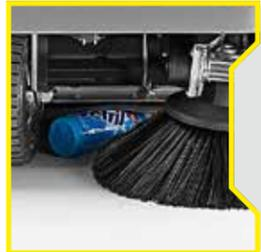
A bulk waste flap is installed in front of the brush and easily opened from the driver's seat. It allows the broom to pick up even bulkier debris.
