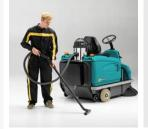
The RIDER 1201 sweeper (EB version only) is also available with a vacuum cleaner kit. Designed for cleaning under tables, chairs, and other recesses or to reach shelving and raised surfaces.
