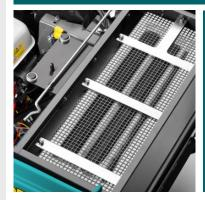
With an innovative structure, large filtering area and up to 99.9% filtration efficiency, the Multipocket Filter® delivers clean air back into the environment and guarantees filter performance that lasts over time. The filter is also washable, resistant to water and oil, self-cleaning and 3888 easy to maintain.
