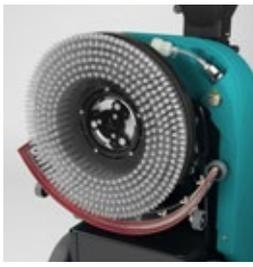
Cleaning solution is delivered directly to the center of the brush, ensuring even distribution. The 360 mm brush enables cleaning even in the most congested spaces.
