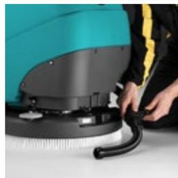
Complete access to the tanks makes after use maintenance easy. The recovery tank can be quickly emptied thanks to the wasterwater tube which is fitted with a valve, and the solution filter is simple to check and clean.
