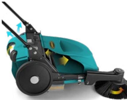
The lateral wheel of the sweeper in addition to activating the main brush, also activates a drive shaft connected to a fan. The ratio between the wheel and drive shaft creates strong suction, which picks up dust and channels it towards the filter. This manual sweeper with an integrated vacuum and filtration system, which does not require motors, guarantees simplicity, affordability and is an eco-friendly choice.
