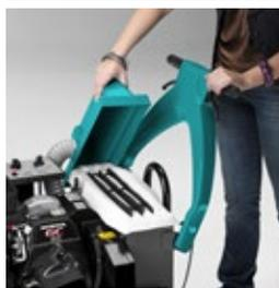
Fine dust is filtered through a polyester bag filter, with a 99,9% filtration rate. This filter has a much longer life span than a traditional filter and can be easily cleaned via the built-in mechanical shaker.
