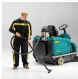
The RIDER 1201 sweeper (EB version only) is also available with a vacuum cleaner kit. Designed for cleaning under tables, chairs, and other recesses or to reach shelving and raised surfaces.
