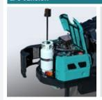
The petrol version (Magnum HGK LPG) can also be used with LPG gas, meaning it's possible to work in both interior and exterior environments with the same machine.
