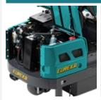
All the internal mechanical parts of the sweeper are easy access for simple maintenance operations, all the rear, side, and upper panels completely open. The batteries (EB EVOLUTION version) can be changed quickly and simply.
