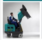
The hopper is positioned at the front of the machine and can be lifted, via a hydraulic high dump system, to a maximum height of 1.565 mm. The hopper is floating, and self regulates to facilitate the pick up of bulkier debris.
