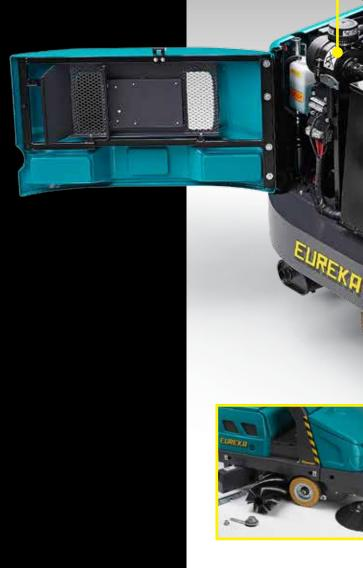
All parts, motors and engines are easily accessible for servicing as side, upper and rear panels can be fully opened. Batteries (EB version) can be replaced easily and quickly thanks to a battery trolley mounted on rolling bearings. This slides out for ease of use.
