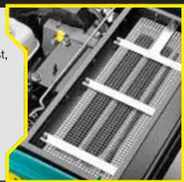
The battery operated version boasts a superior running time, for extra productivity. Maintenance access is convenient as well. The top lifts up to expose the engine or the battery compartment as well as motors and other service areas.
