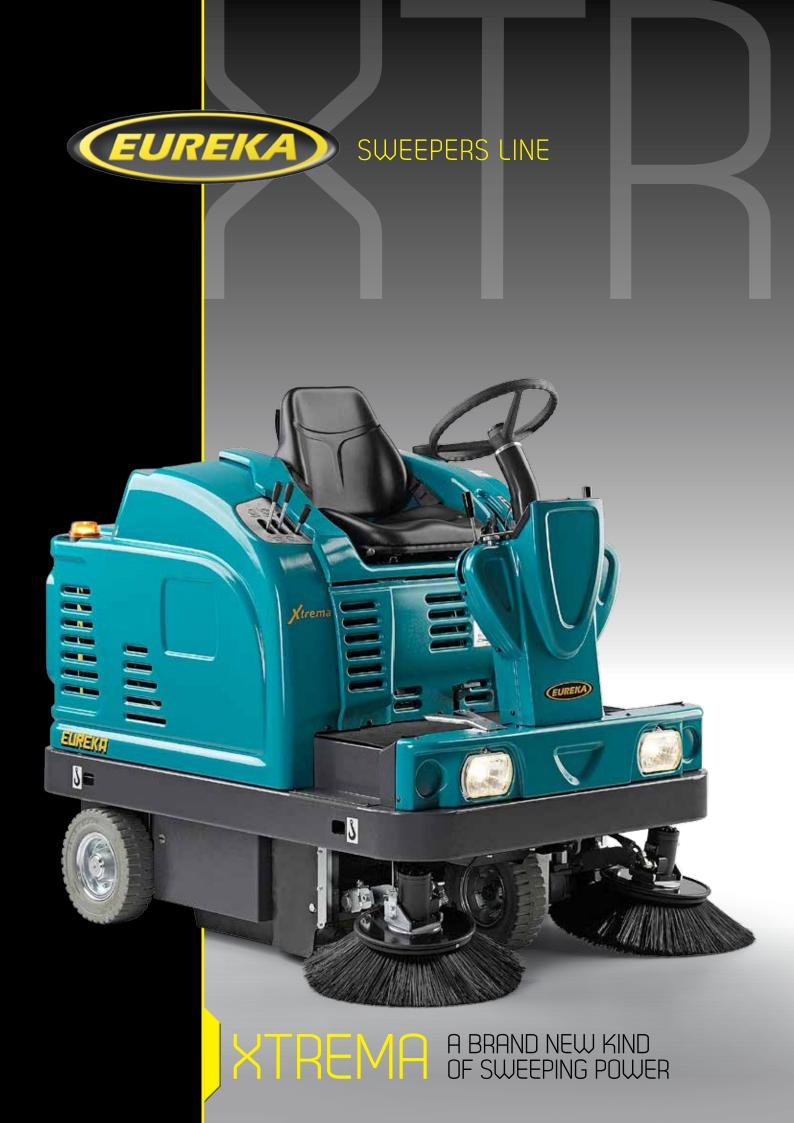
THE XTREMA IS A COMPACT. COMPLETELY HYDRAULIC **CONTROLLED HIGH DUMP** SWEEPER DESIGNED AND MANUFACTURED BY EUREKA TO SWEEP CONGESTED AREAS AS WELL AS LARGE FLOOR SPACES. IT HAS A MAIN BRUSH WIDTH OF 800 MM, A TOTAL SWEEPING PATH OF 1.400 MM AND A CLEANING CAPACITY. AT FULL SPEED, OF 12.600 SQ/M/H.
