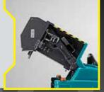
Xtrema is equipped with a polyester bag filter which is particularly efficient for the retaining of fine dust, and has a much longer lasting life than other traditional filters.
