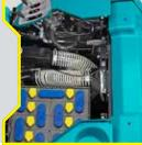
Strong hydraulic drive system, variable speed controlled up to 9 Km/h, by means of two pedals (fwd & rev)
