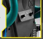
Waterflow adjusting knob and dosing system pump connection.
