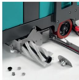
The components of the machine that require inspection and maintenance can be easily removed, without using tools.
