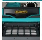
Antistatic filter, washable, with an automatic shaking system. Delivers high performance filtering that is maintained over time.
