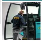
Security and driving comfort are increased with the pressurized, air-conditioned cabin. Offers maximum protection to the operator and provides full visibility of the right side brush.
