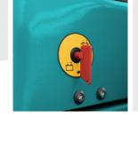
Numerous devices, such as the seat sensor and current cut-off switch. ensure operation with maximum operator protection.
