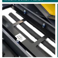
With an innovative structure, large filtering area and up to 99.9% filtration efficiency, the Multipocket Filter® delivers clean air back into the environment and guarantees filter performance that lasts over time. The filter is also washable, resistant to water and oil, self-cleaning and easy to maintain.
