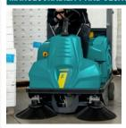
The car-like steering, the great visibility offered and the turning radius of only 1,050 mm make the Rlder Lift an extremely agile and versatile machine.
