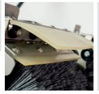
Located directly beneath the brushes, the channel catches any drips of solution and facilitates thorough vacuum drying. Polyurethane spray guards prevent upward splashing.
